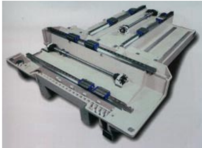
Figure 45 : Guidages de la machine MIKRON VCP 1000
